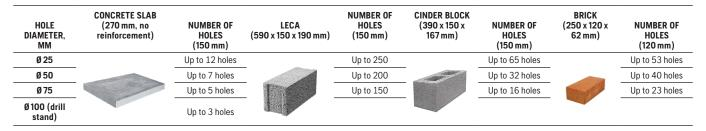
\* Drilling results may vary depending operator skills, ambient conditions, type of material and the quality of the diamond core drill bit and should be viewed as indicative only. For this chart a DM 540i and a BLi300 battery was used, running the battery from fully charged to empty, with an Elite-Drill TW core drill bit for wet drilling.
