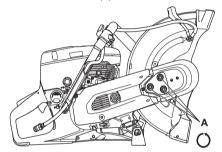
Wiggle the blade guard (E) up and down 3-5 times, and then tighten the nuts (A) with the combination spanner.
