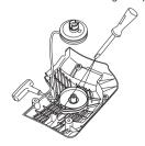
Remove the recoil spring by turning the starter over and loosen the hooks, with the help of a screwdriver.
