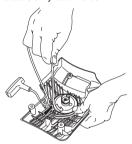
Remove any remnants of the old starter cord and check that the return spring works. Insert the new starter cord through the hole in the starter housing and in the cord pulley.
