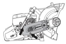
Replace the drive belt. Turn the belt tensioner (B) to position "1" to tighten the drive belt.
