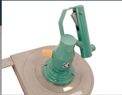
Motor with preventive switch lock
