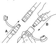
**CAUTION!** Two hose kits can be connected when hose lengths exceeding 18 m are required. Do not connect more than two kits as the couplings cause large power loss. See the Technical data.
