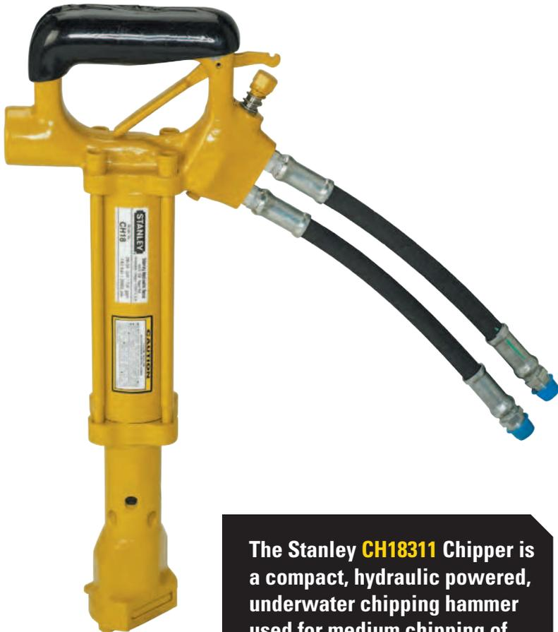
The Stanley **CH18311** Chipper is a compact, hydraulic powered, underwater chipping hammer used for medium chipping of concrete, masonry and rock.
