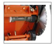
**LOW MAINTENANCE**The IntelliSeal blade shaft system allows for a minimum of 250 maintenance-free hours without daily greasing of bearings.
