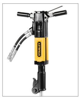
The rugged, lightweight and powerful construction of the BR50 T handle and BR50S anti vibration handle breakers makes them ideal for use in the 35 - 65 pound class. Designed for light to medium duty operation, they excel at curb and sidewalk demolition, asphalt cutting, and are popular for ground rod driving with electric utilities.
