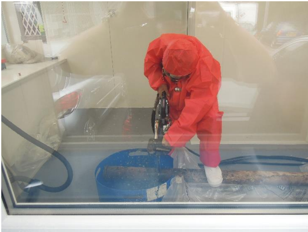
PowerGrit tested for asbestos cutting
