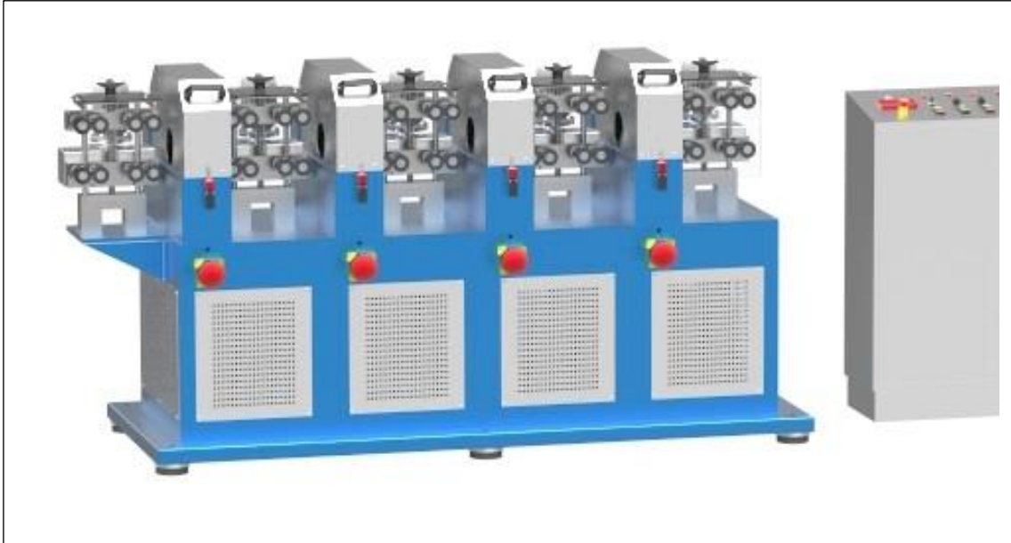
Machine shown with 8 wheel auto self centering feeds attached
